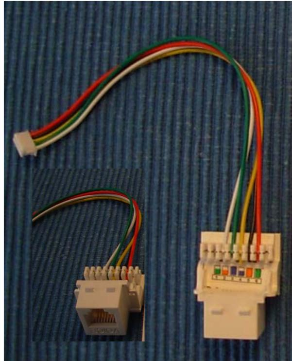
Above is a completed adapter. The clear plastic cover has not been restored. The red wire is attached to the rightmost of the active terminals. The attached label says this is terminal 6, but we are considering it number 1. From a slightly different angle (inset) one can see that it is the rightmost active terminal when looking from the front, and with the clip-tab pointing upward.
