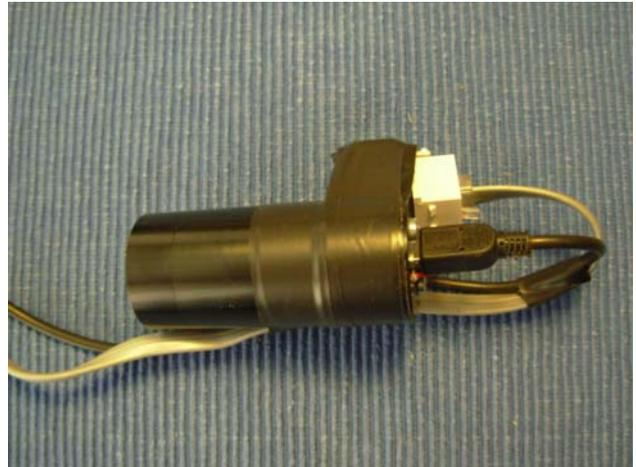
The finished product (above) is an RJ-12 jack connected to a Lodestar-type connector. Here, a standard autoguider cable coming from the jack is taped to the USB-Mini connector to share strain relief on the cables. These cables are then taped to the side of the Lodestar to further eliminate any strain on the connections themselves.
